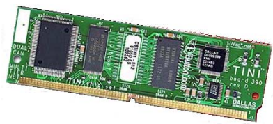
Fig. 3. TINI TM board at SIMM card format
